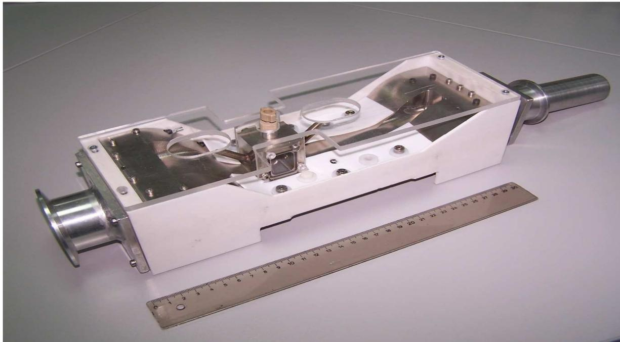
Picture of a previous generation flat DMA, where the sheath gas inlet and outlet, and the insulator box (white color) can be seen. The upper part includes the Ionization chamber.
