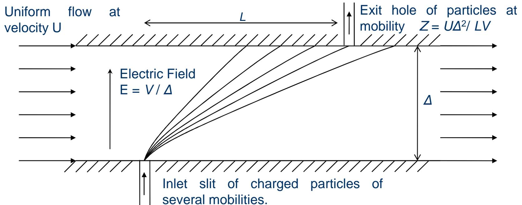
A Differential Mobility Analyzer (DMA) is an instrument that separates ions as a function of their electrical mobility, just as IMS. The main difference between both instruments is that the DMA separates ions in space, while IMS does so in time (inefficient duty cycle). As a result, a DMA has a two orders of magnitude sensitivity gain over an IMS.
